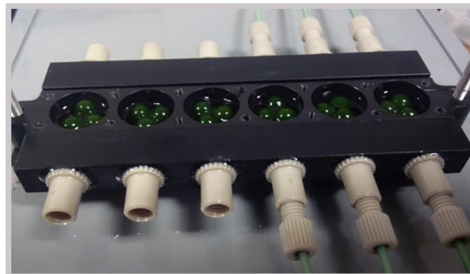
↑ Figure 4 — Embedded and immobilized algae (green beads) in the photosystem II fluorescence sensor. The system allows six parallel flow cells.
