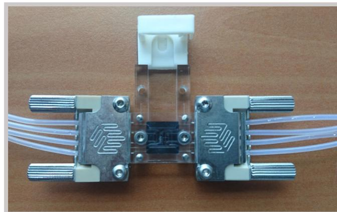
↑ Figure 1 — The final multiplex aMZI nanoimmunosensor chip (middle) with connecting optics (right and left) and the superimposed microfluidics connection (middle to top).
